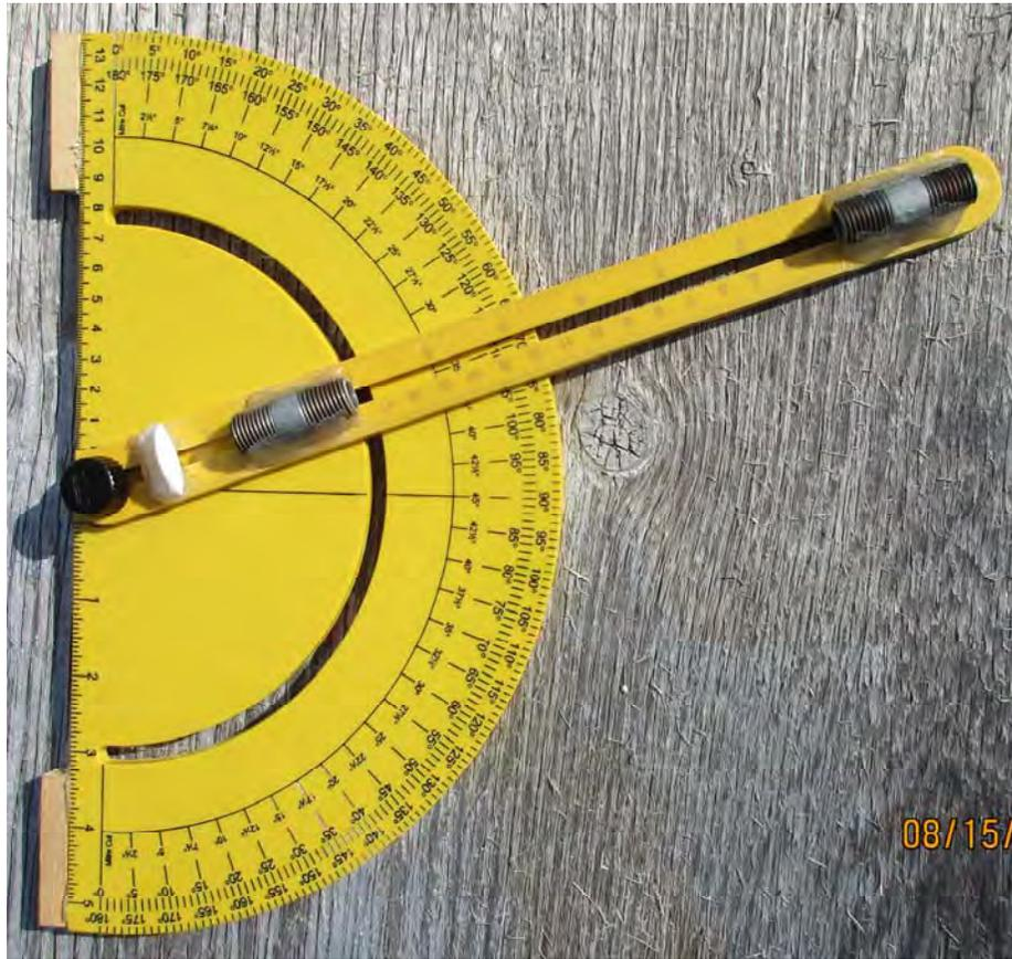
The basic protractor was purchased from Harbor Freight tools. The sun makes a shadow of each round pipe that falls onto the white surface. When both shadows of the sun align, then the reading is taken.
